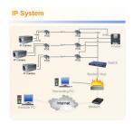
In the IP world, each network camera captures an analog image but immediately converts it to digital inside the camera. Some digital processing can happen right at the camera, such as compression and motion detection. The digital video stream is then broadcast over the IP
